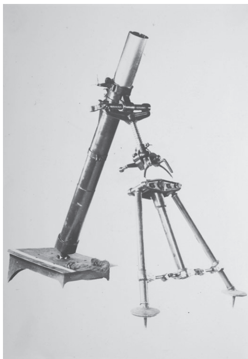
British ML 3-inch mortar (81 mm), also known as 'mortar of 8'. Source: NIMH / Foto-afdrukken Koninklijke Landmacht.
