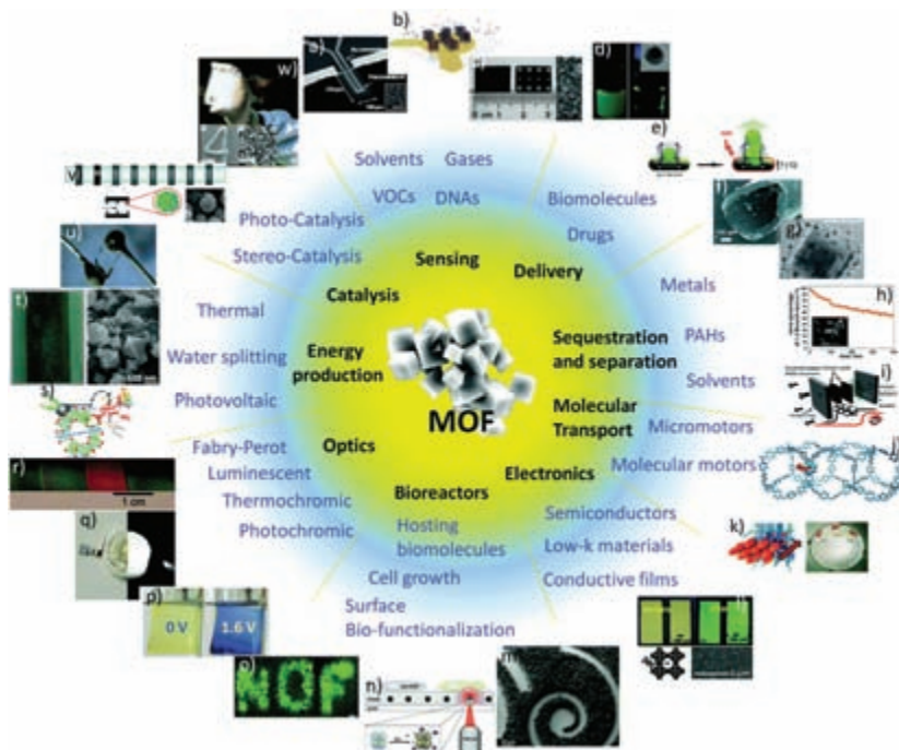
Figure 3. MOF-based devices a) MOF-based piezoresistive microcantilever, b) MOF-deposited gold QCM electrodes, c) HKUST-1 film on aluminium electrodes, d) magnetic manipulation of \text{Fe}_3\text{O}_4 -loaded ZIF-8, e) near infrared-induced drug release from gold nanorod-loaded MOF, f) MOF-5-coated fused-silica capillary, g) HKUST-1-coated silica magnetic bead, h) MOF-5 magnetic framework composite and the uptake of benzantracene, i) HKUST-1 incorporated micro-separator assembly, j) porous aromatic framework structure with a highlighted p -phenylene rotor, k) projection of a MOF-peptide 'boat' around the Petri-dish, l) TCNQ molecule entering a HKUST-1 film devices, m) MOF patterns created by UV lithography, n) photosensitive MOFs for cell activation, o) cell activation by irradiation-induced selective release of NO from MOF devices, p) MOF thin film-based reversible electrochromic device, q) MOF-based white emitting LED, r) ZIF-8-based Fabry-Perot interferometer, s) photoexcited organic linker induced electron transfer from the linker-to-cluster charge-transfer mechanism, t) MOF-coated doctor bladed \text{TiO}_2 -MWCNTs composite, u) gold electrodes attached to a single MOF crystal, v) magnetic framework composite immobilized into a microfluidic catalytic system, w) HKUST-1 films on a photolithographed copper plate. Chem. Soc. Rev. 2014, 43, 5513–5560, and references therein. Published by The Royal Society of Chemistry.
