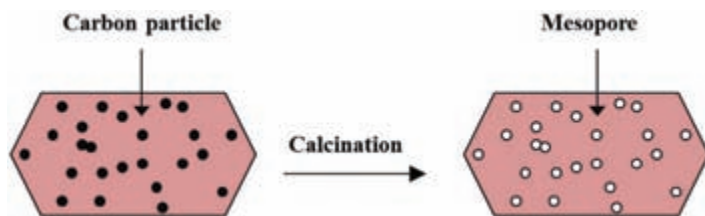
Figure 7. Synthesis of hierarchical zeolite by carbon nanoparticles.
